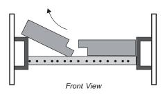
Important: push both baffle bricks so they are tight against the side walls.
